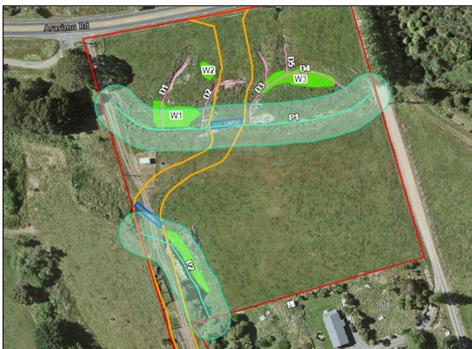
Figure 6b: 10 m setbacks from Streams P1 and P2 at the northern end of the site (turquoise polygons). Streams are shown with a turquoise line, wetlands with a green polygon, drains with pink lines. The extent of earthworks for the new access track is shown with an orange line, and the extent of the culverts with blue lines.
